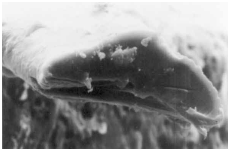
FIGURE 10-13 A scanning electron photomicrograph of the cross-section of a nylon fiber removed from a sheet used to transport the body of a murder victim. The fiber, associated with a carpet in Wayne Williams's home, was manufactured in 1971 in relatively small quantities. Courtesy Federal Bureau of Investigation, Washington, D.C.
