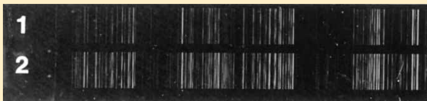
FIGURE 2 A comparison of paint chips 1 and 2 by emission spectrographic analysis. A line-for-line comparison shows that the paints have the same elemental composition.
