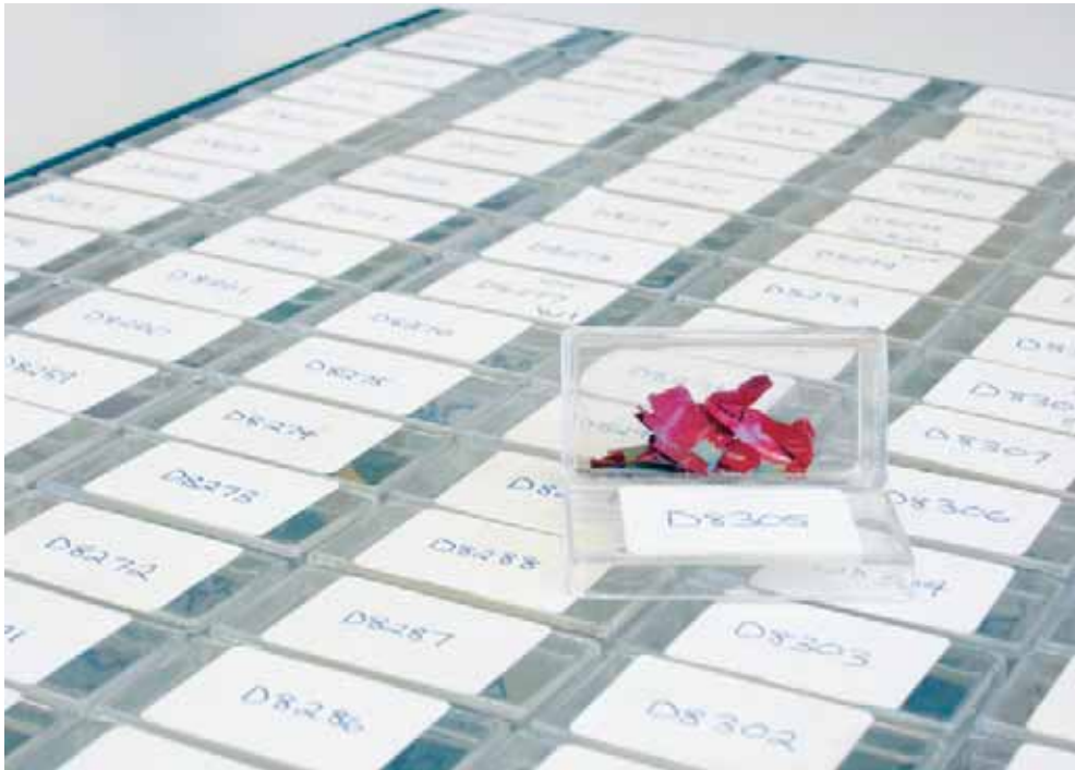
FIGURE 11-13 A crime laboratory's automotive paint library. Paints were collected at an automobile impound yard and then cataloged for rapid retrieval and examination. Courtesy Gavin Edmonstone, Centre for Forensic Sciences, Toronto, Canada
