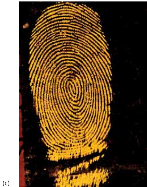
FIGURE 14-18 (a) Latent fingerprint visualized by cyanoacrylate fuming. (b) Fingerprint treated with cyanoacrylate and a blue/green fluorescent dye. (c) Fingerprint treated with cyanoacrylate and rhodamine 6G fluorescent dye. (d) Fingerprint treated with cyanoacrylate and the fluorescent dye combination RAM. (e) Fingerprint visualized by the fluorescent chemical DFO. (f) Fingerprint visualized by Redwop fluorescent fingerprint powder. (g) A bloody fingerprint detected by laser light without any chemical treatment. (h) A bloody fingerprint detected by laser light after spraying with merbromin and hydrogen peroxide. (a) Courtesy North Carolina State Bureau of Investigation, Raleigh, N.C. (b) Courtesy 3M Corp., Austin, Texas (f) Courtesy Melles Griot Inc., Carlsbad, Calif.
