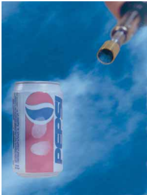
FIGURE 14-14 Super Glue fuming a nonporous metallic surface in the search for latent fingerprints.
