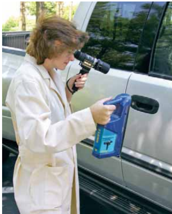
FIGURE 14-11 Using a Reflected Ultraviolet Imaging System with the aid of a UV lamp to search for latent fingerprints. Courtesy Sirchie Finger Print Laboratories, Inc., Youngsville, N.C., www.sirchie.com
